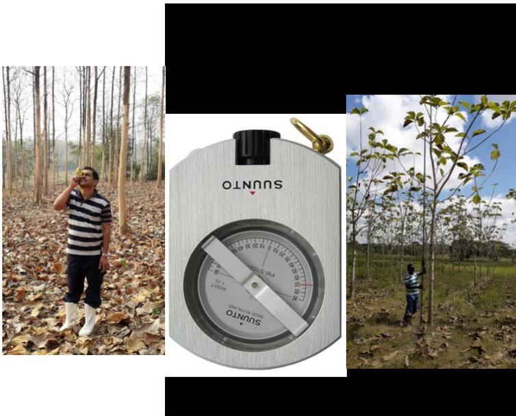
Figure 2.3. Total Tree height was measured by hypsometer and a pole, used instrument of sununto meter is shown in above
