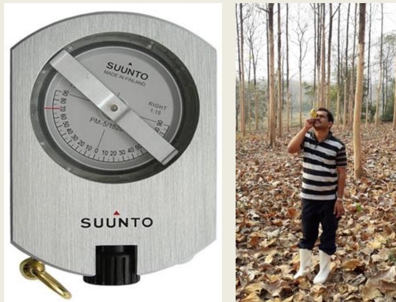
Figure 1.2. Total Tree height was measured by hypsometer, used instrument is shown in left side
