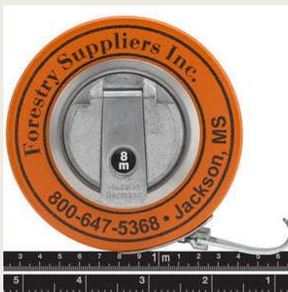
Figure 1.1 Diameter tape used for the inventory
