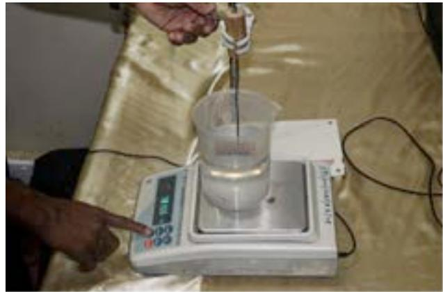
(a) Wood samples for density measurement taken from pith to bark. (b) Volume of wood sample
